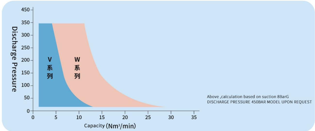
\*The above parameters are calculated based on 8barg inlet pressure;
